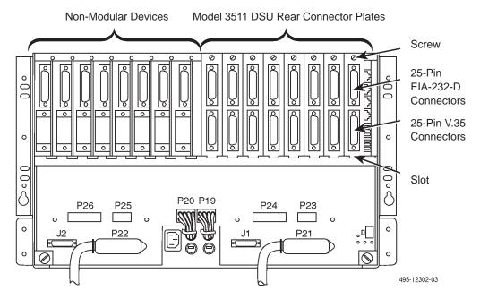
Figure 2. Rear View of the COMSPHERE 3000 Series Carrier
